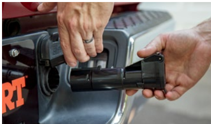
Insert Echo between the vehicle and trailer
