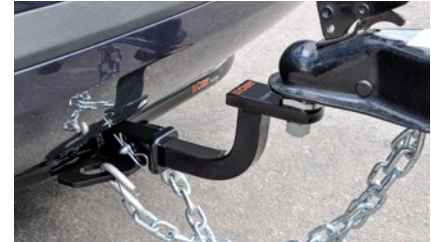
Multiple drop and rise options accommodate various vehicle-trailer combinations
