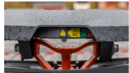
Three-position coupling indicator clearly shows coupling status
