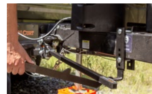
Adjustable brackets and lift handle provide fixed support
