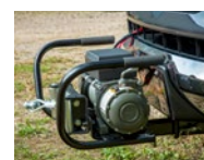
Allows a winch to be easily attached to a receiver
