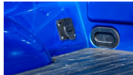
10' routes socket closer to truck cab
