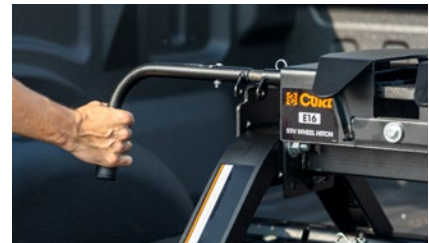
Single-handle operation with auto-lock for easy, secure coupling
