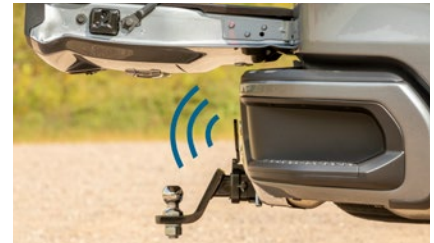
Prevents deployment of inner tailgate panel when ball mount is installed
