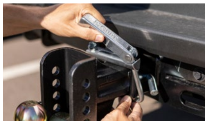
No-tool installation and easy-to-adjust clamp lever (clamp-style)
