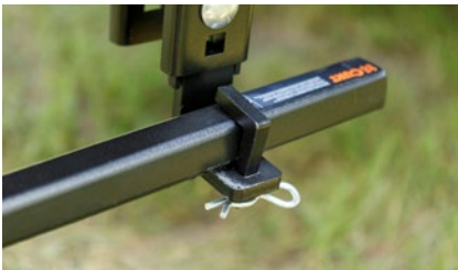
Two points of sway control use friction to keep trailer aligned
