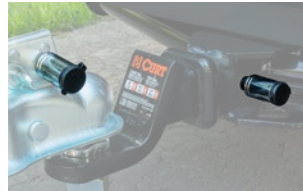
Watertight dust caps prevent internal corrosion
