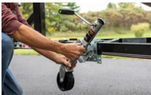
Swivel bracket allows jack to fully swing up during travel
