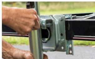
Heavy-duty pull-pin locks jack securely in place
