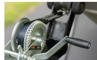
Straps made from 2" wide, no-stretch nylon web
