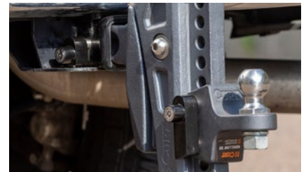
Locks replace standard clips and hitch pin for increased security
