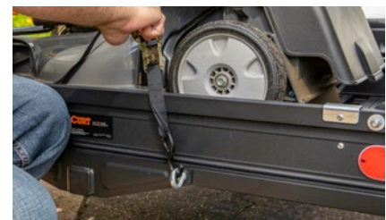
Six integrated eye bolts for secure attachment of straps or other tiedowns
